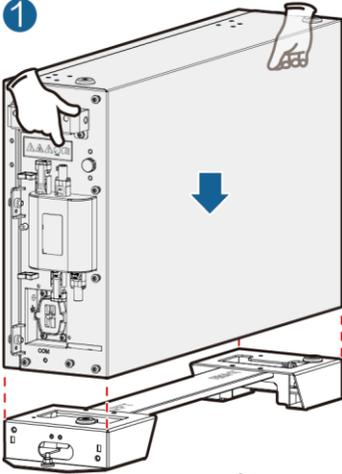
Align the first battery expansion module with the support on the floor support.
