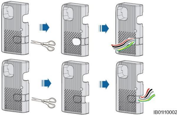
Cut a cable hole based on the cabling mode, and route external cables through the cable hole.
