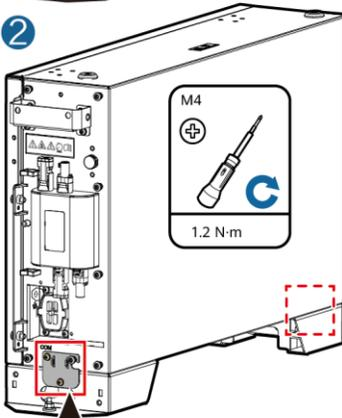
Install the connecting pieces on both sides and tighten the four screws.
